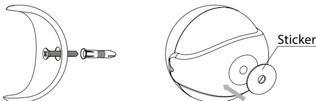
2. Insert the device into the holder.
