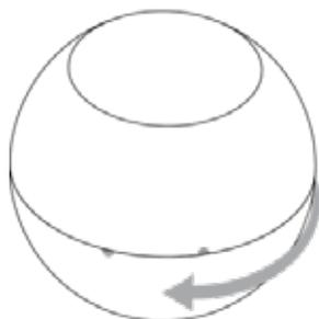
2. Remove the battery blocker.
