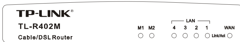
Figure 2-1: Front Panel sketch
