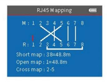
TDR helps to pinpoint where cabling faults occur. This speeds up fault finding as well as minimising disruption and potential damage to fixtures and fixings.
