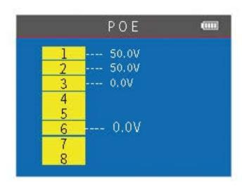
Detect Ethernet network for POE (Power over Ethernet) existence and to know which pair is providing power and with voltage information.
