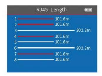
Utilises TDR to accurately measure cable length with visual length graphics and provide distance to fault information.
