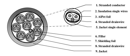
Each pair individually shielded with Beldfoil® aluminium-polyester shield. Individual pairs with numbered FRNC jacket.
