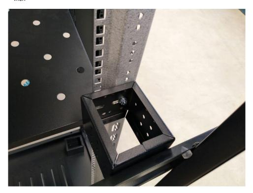
4. Fix the vertical rails with screws
