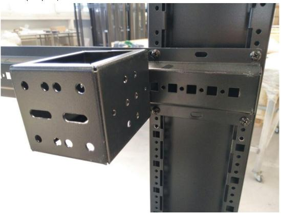
3.Fix the two cubs on one horizontal rail, then fix the vertical rails on the cubs to make sure 19 inch
