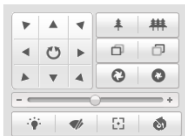
Figure 4-3 Panou de control PTZ
