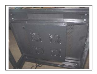
Carefully attached the supplied 'Fan Tray' to the top of the inner surface of the installed perforated roof.
