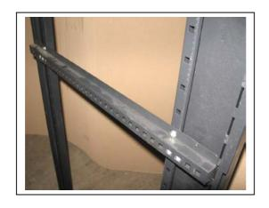
Please attach 'Cage nuts' to horizontal profiles <u>before</u> bolting to the frame using holes 4 & 5 (600mmX600mm, 600mX800mm Cabinets only)
