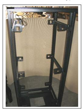
Carefully install the supplied 'Box Spacers (x12 in total) on the front and rear points of the previously installed 'horizontal support bars (see item 6 on page 4).
