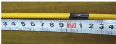
Pic 3: the length of stripped fiber cable
