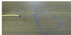
Pic4: fiber after stripping
