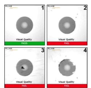
**End-face Defects -** Visual defects are one of the most common causes of latent failures. Scratches, pits, and hips in the ferrule end-face can change over time, becoming more pronounced and migrating to critical areas of the fiber core, thus affecting Performance. They are also a prime source for deposits of dust, moisture, and other contaminants.
